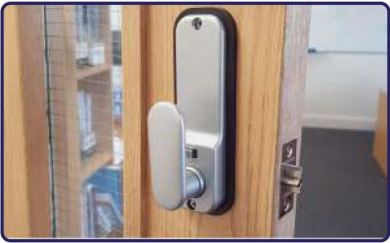
BL2901 ECP (Holdback) Anti-ligature knob keypad with a tubular latch and internal paddle handle with holdback function
